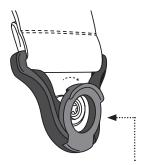
Spring-loaded latch automatically locks onto instrument
