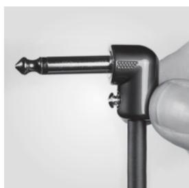
With the included screw driver, loosen set screw on the plug to allow clear entry to the plug barrel. Push cable into the open plug end with a "twisting" motion until it is fully seated.
