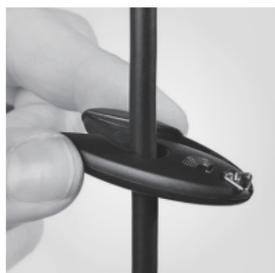
Using included cable cutter, cleanly cut cable to desired length avoiding any loose or overhanging strands of shielding.
