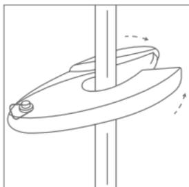
Cleanly cut cable to desired length avoiding any loose or overhanging strands of shielding.
