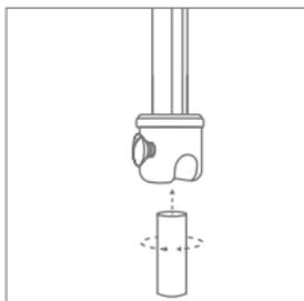
Loosen set screw on plug to allow clear entry to plug barrel. Push cable into open plug end with a "twisting" motion until it is fully seated.
