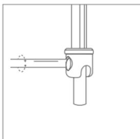
Completely tighten set screw.
