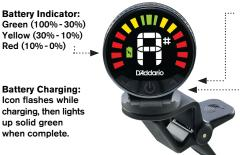
Calibration Buttons: adjust tuner calibration from 415 to 465Hz.
